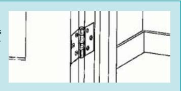
doing any planing. After years of use, hinges become worn so that the pins are slack and the door drops. In this case, fit new hinges, or, as a cheaper alternative, swap old hinges, the top with the bottom, which will reverse the wear on the pins. Finally, replace the door and check to see that it no longer sticks.
